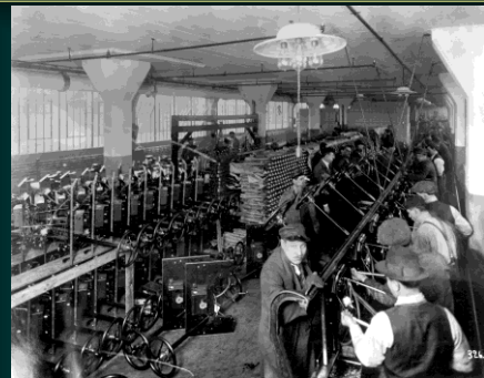
Assembly line for Model T dashboards, 1914
