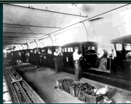
Assembly line installation of tops on Model T bodies, 1915
