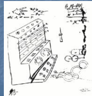
A 1624 sketch Schickard made of his calculator
